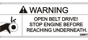
PART NO. 303517 LOCATION: LH Side of Rear Surface of Mower Deck
